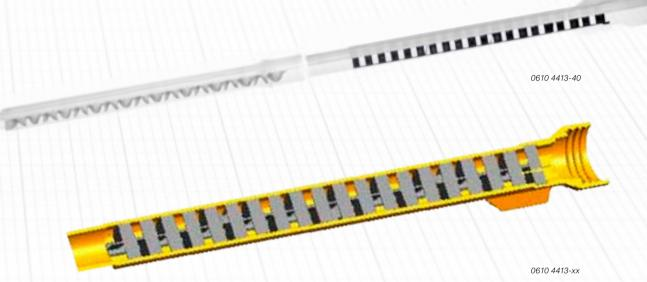
The QUADRO™ High Flow mixer was developed for dispensing large amounts and high-viscosity products. The patented QUADRO™ mixing technology uses a large mixer diameter and open mixer structure to minimize the required application pressure.
