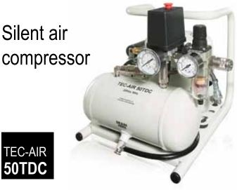
The tec-AIR 50TDC is an almost silent, compact, air compressor. It weighs just 21 kilos (46lbs), and comes complete with a robust tubular carrying frame. It is rated at 50 l/min (2.15cfm) and works to a maximum pressure of 8 bar (120psi). It is capable of operating up to two tec 6100 or tec 7100 applicators or one tec 6300 or tec 7300 spray applicator intermittently for small area coverage. It can also be used with most other pneumatic tools such as staplers, air brushes and tyre inflators.
