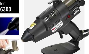
Extremely robust 43mm (1¾") spray glue gun with power-on light. Designed for industrial use, it sprays hotmelt at any angle with adjustable spray pattern. A non-toxic adhesive spray system, it covers large areas and applies hotmelt to heat sensitive substrates without damage. 7 bar (100psi) 85 l/min (3 cfm) air supply required.
