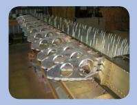
Permabond 910 methyl-based cyanoacrylate adhesive is approved by Boeing (to spec BMS5-36D Type I). Lightweight aluminium wing spars are bonded during construction of aircraft wings.
