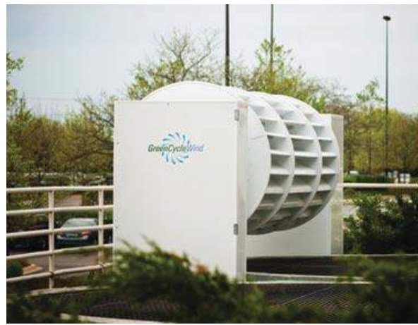
Fig. 3: LORD Corporation's new Maxlok adhesive is utilized in the construction of the dual source Green Cycle Wind turbine to improve joint design, reduce weight and reduce assembly design.
