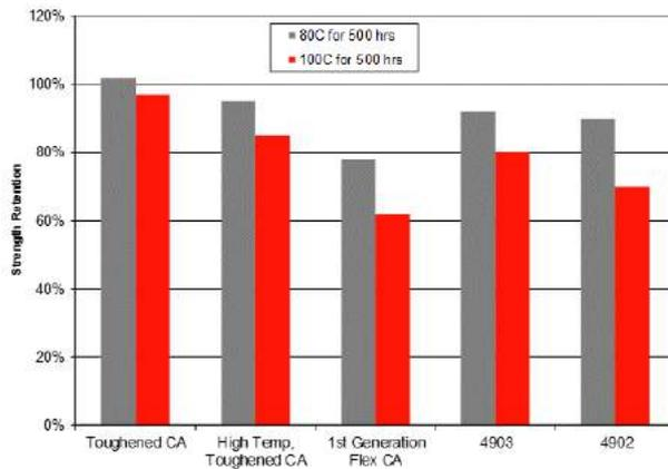
**Figure 3 – Heat aging stability of cyanoacrylates for 500 hours of aging.**
