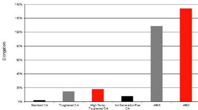
**Figure 4 – Bulk elongation properties of various cyanoacrylates.**
