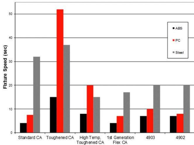
**Figure 1 – Fixture speed of cyanoacrylates on various substrates.**
