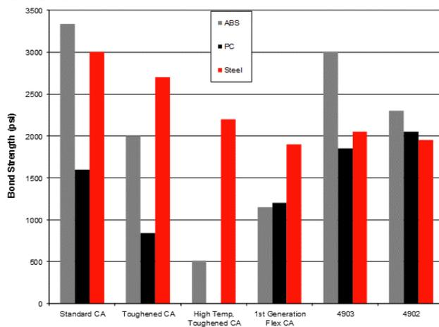
**Figure 2 – Shear strengths of cyanoacrylates on various substrates.**
