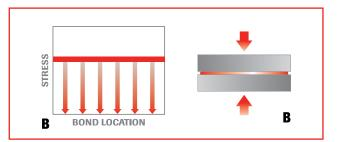
**COMPRESSION STRESS DISTRIBUTION:** When a bond experiences a compressive stress, the joint stress distribution is illustrated as a straight line. The stress is evenly distributed across the entire bond.
