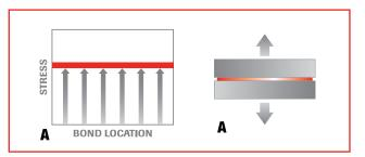
**TENSION STRESS DISTRIBUTION:** When a bond experiences a tensile stress, the joint stress distribution is illustrated as a straight line. The stress is evenly distributed across the entire bond. Tensile stress also tends to elongate an object.
