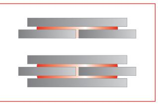
**STRAP JOINT (SINGLE OR DOUBLE):** A strap joint is a combination overlap joint with a butt joint.
