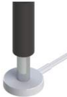
Figure 6. BlueWave® LED Prime using a 8-mm lightguide, measured directly on the surface of the radiometer
