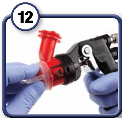
12 Re-attach the same atomizing head or when necessary replace with a new one.
