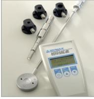
ACCU-CAL<sup>™</sup> 50 Radiometer Ideal for process monitoring
